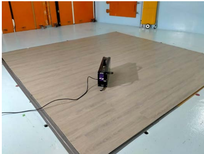
Figure 2.1: Sample installed on chamber floor with tapping machine
