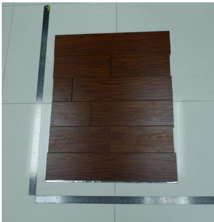
Photo 2. Eprouvette d'essai/ *Test specimen – Laminate Flooring –*
